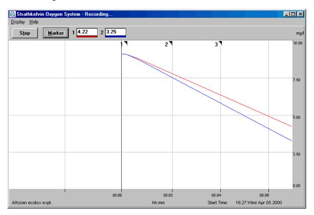
The main part of the screen is the same as in Set-up and displays the oxygen traces. However, you will notice that the time and date at which recording started has been inserted below the recording area. On the toolbar, the **Start** button has been replaced by a **Stop** button, and the previously greyed out **Marker** button is now enabled. The **Marker** button allows you to record events during a respiration run, such as the addition of an inhibitor to the respiration chamber.
